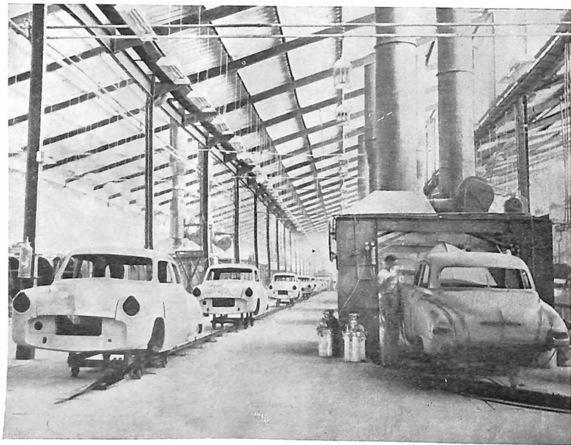
A Motor Car Factory in Calcutta. Photograph shows car bodies receiving the final coating of colour
