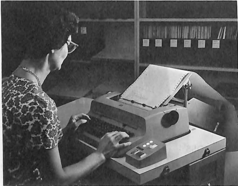
FIGURE 6.1 The JOSS Console, Consisting of a Modified IBM Selectric Typewriter and a Control Box
