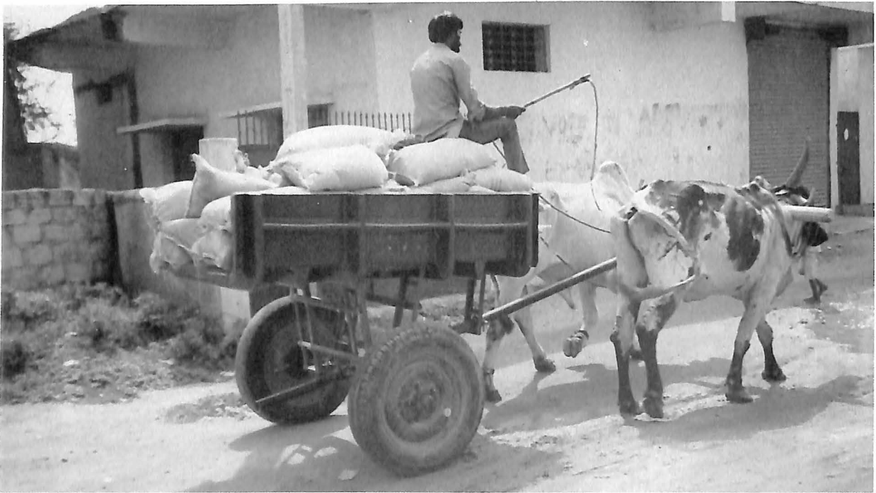
An improved bullock-cart for 1.5 tonnes pay-load.
