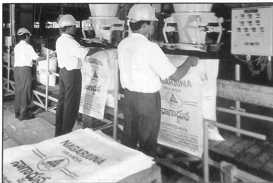
Inside view of bagging section of Nagarjuna Plant.
