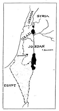
This canal would start right up towards the headwaters of the Jordan, in Israel, and would run out westwards, taking the water out of the Jordan basin altogether, into the coastal plain and on into the Negeb.
