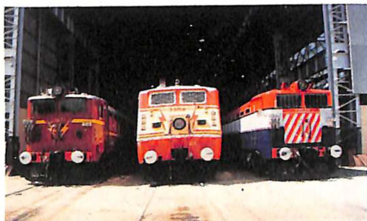
WAG-5, WAP-1 and WAG-7 types of electric locos built by CLW.
