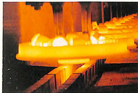
Cast steel BOX 'N' wheels on conveyor inside hot wheel kiln, W&AP.
