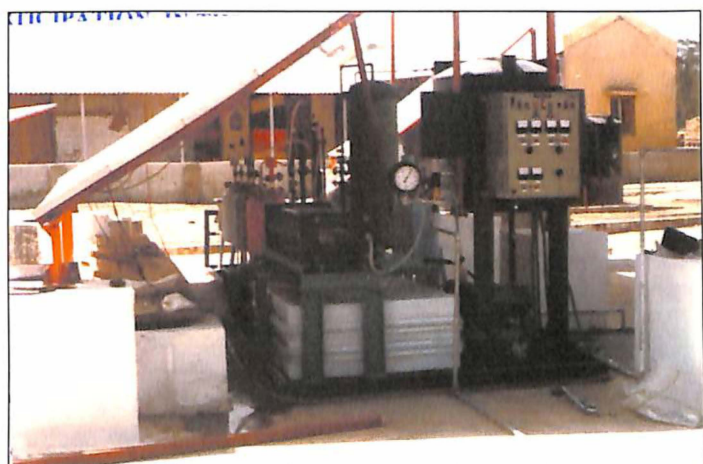
Reverse osmosis demonstration plant (Capacity : 5 kilolitre per day) that runs on solar energy
