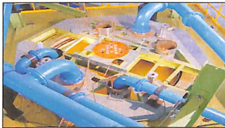
Pool Hydraulics – Prototype Fast Breeder Reactor 1/4th Model
