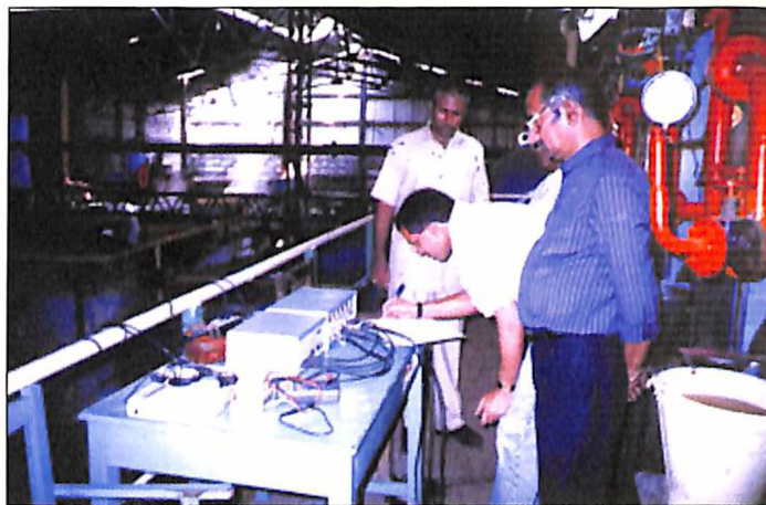
Radiotracer testing in action in a sugar mill
