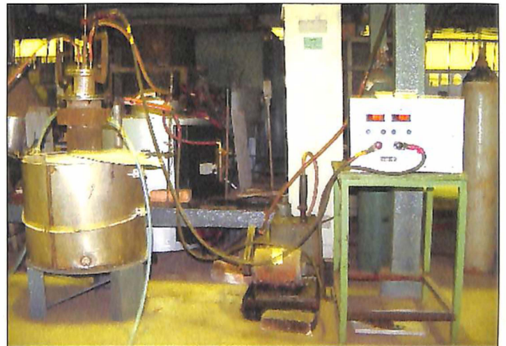
Electrolytic setup used for the extraction of boron
