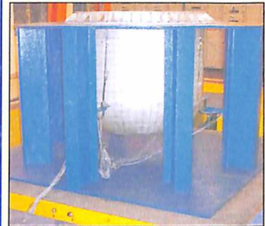
Seismic tests in progress on reactor assembly model
