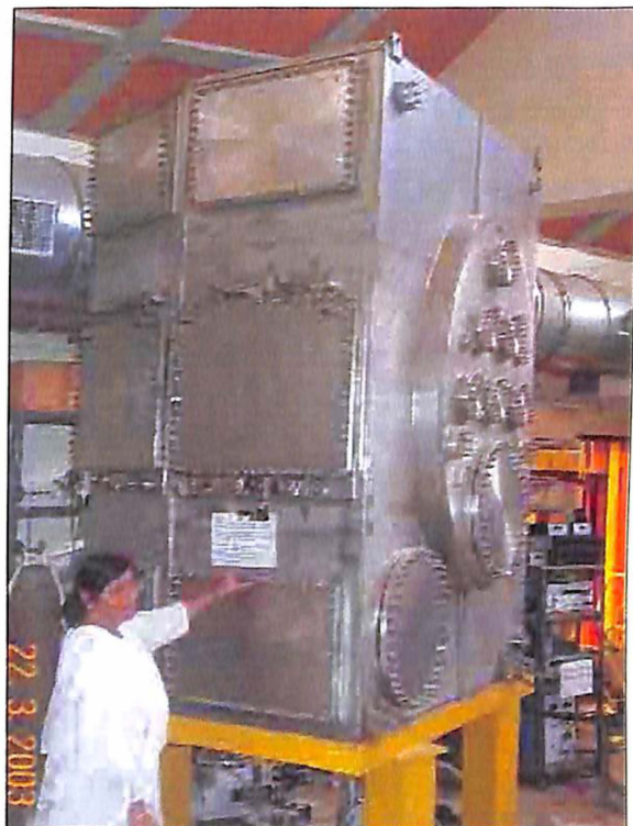
Full scale prototype of steadystate superconducting tokamak (SST-1) cryostat and vacuum vessel
