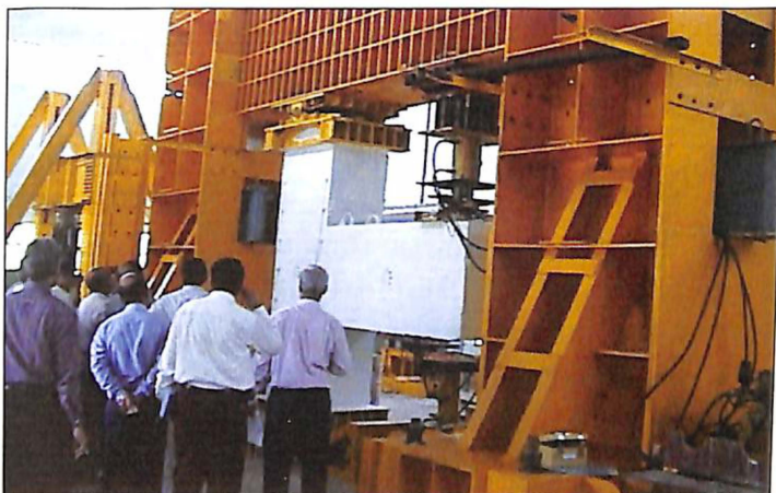
The Test Specimen (beam-column joint of turbine building of 500 MW TAPP 3&4) being tested on the 500 Ton Test Frame built under the BRNS Project, "Experimental and Analytical Evaluation of Nonlinear Behavior of RCC Frame Structures and Joints" at SERC, Chennai
