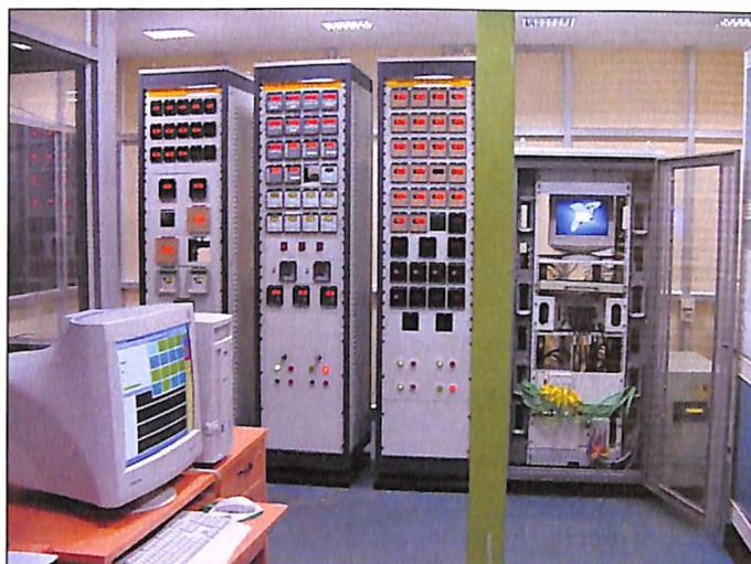
Data Acquisition System for One-Fourth Reactor Assembly Model
