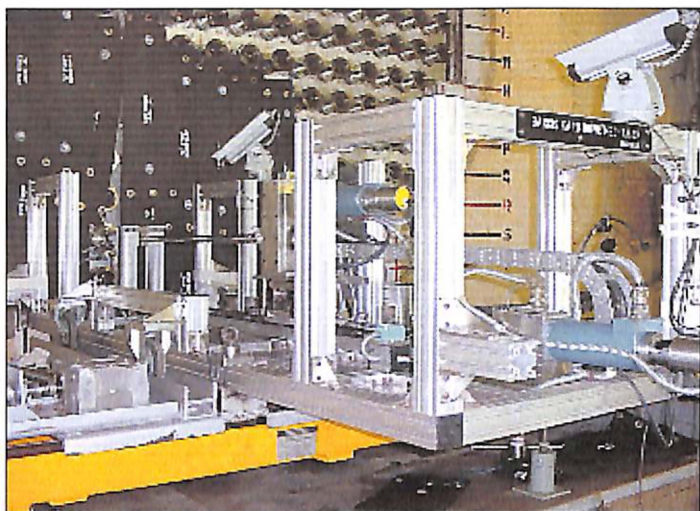
Automated BARC Channel Inspection System (BARCIS) developed for in-service inspection of coolant channels in PHWRs
