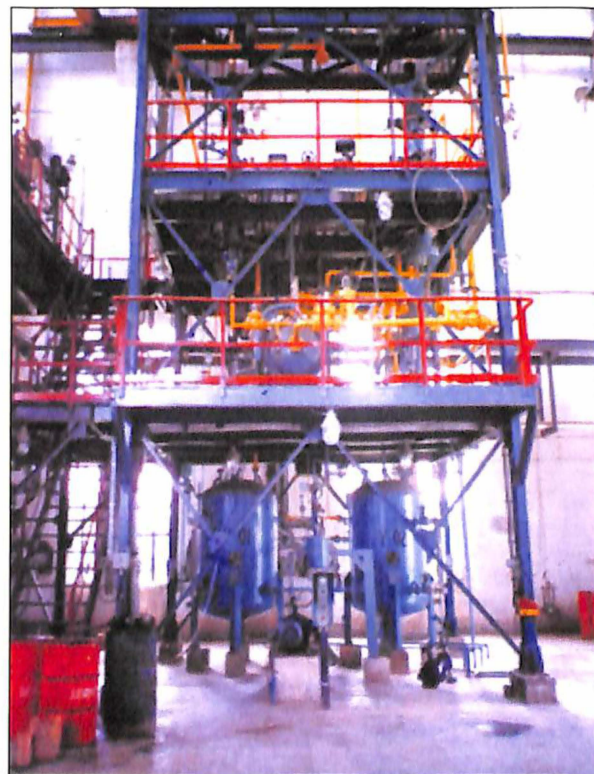
Radiotracer studies being done by BARC on a trickle bed reactor of a factory
