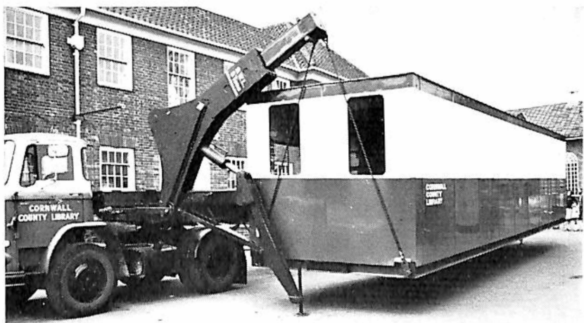
'Where do you want it, mister?' Cornwall County's 'piggy-back' container libraries, which are off-loaded and connected to main services at prepared sites, and offer a telephone service, study facilities, and greater floor and shelf space than a mobile library.
