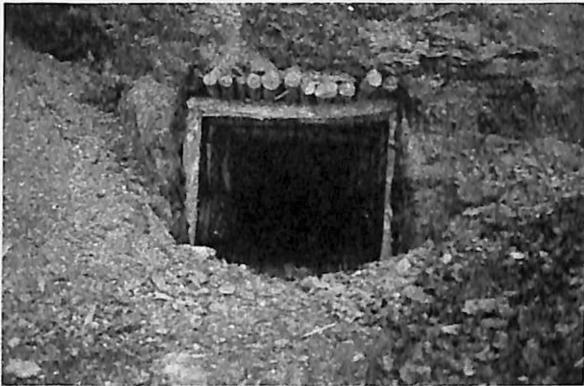
Unscientific, Rat Hole Coal Mining at Namsang, which is generally practised at all the coal mines in Nagaland.
