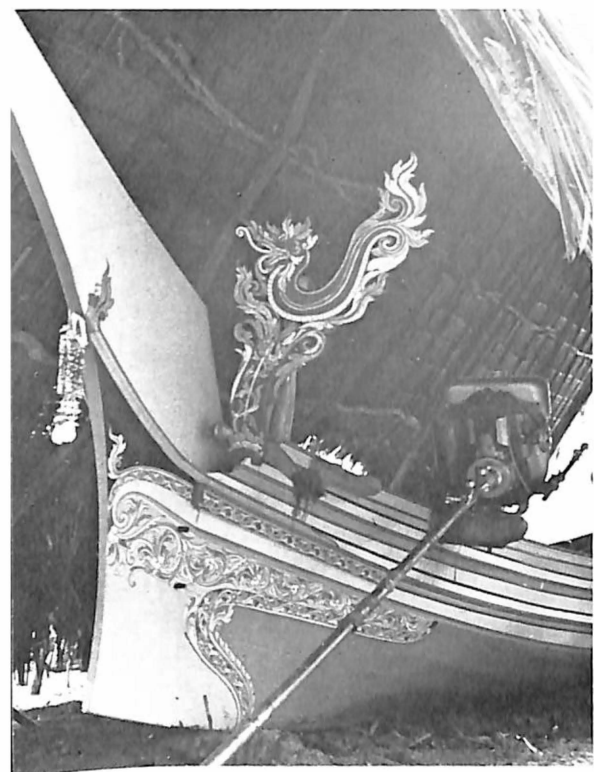
Stern of kolek equipped with "long-tail" outboard motor. Ornate crutch once held its mast when not in use. Garland of flowers is to please sea spirits.
